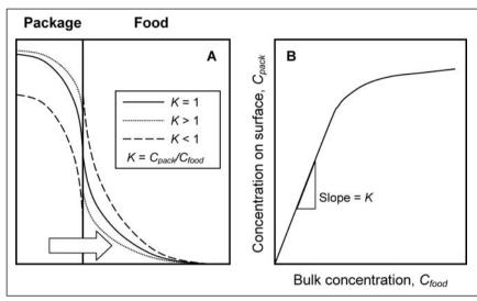
Figure 1 — Effect of interfacial partitioning of molecules on mass transfer between food and packaging materials: (A) migration of package constituents into foods, (B) scalping of food flavor into packaging materials. K is a partition coefficient of a migrant.
