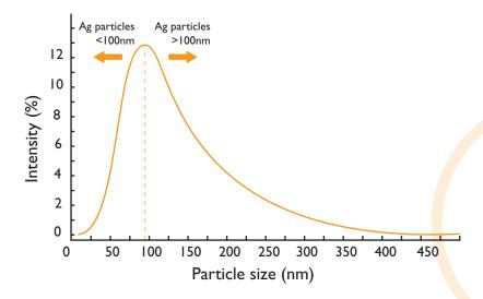
Figure 3.1 Typical Particle Size Distribution Curve for Silver (Ag) Nanopowder Dispersed in Triton X100. The Silver Nano-powder is sold as having a Particle Size of <100nm. The Curve was Obtained using a Malvern Instruments Zetasizer Nano
