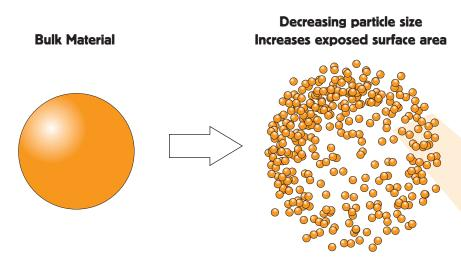
Figure 3.2 Schematic of how the Surface Area Changes as the Particles Become Smaller
