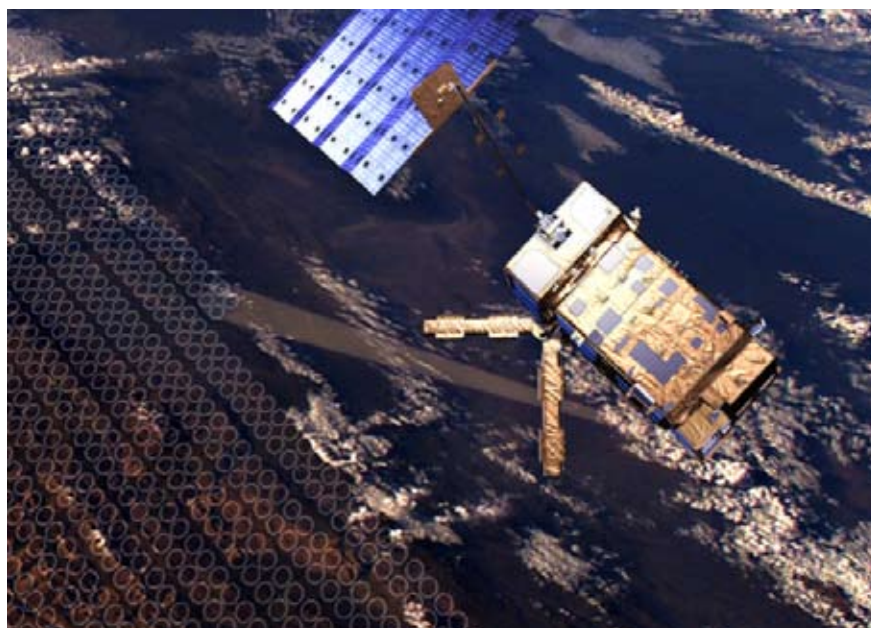
From MetOp's polar orbit, the IASI instrument observes a swath of about 2 000 square kilometres of the Earth (artist's impression)
