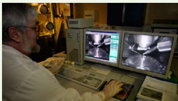
Nuclear forensics at JRC-ITU: operation of the micromanipulator system installed in the Scanning Electron Microscope (SEM) for the transfer of micrometer sized particles
