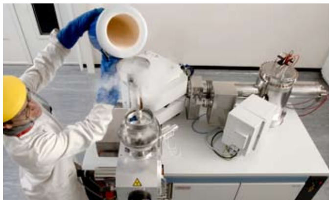
Pouring liquid nitrogen into the thermal ionization mass spectrometer (TIMS) at JRC-IRMM
